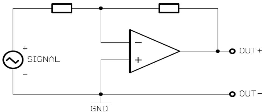
*fig. 3: single ended signal stage*
