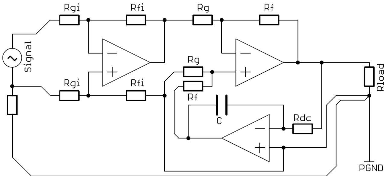
*fig.7 simplified grounding sheme with DC-Servo*
