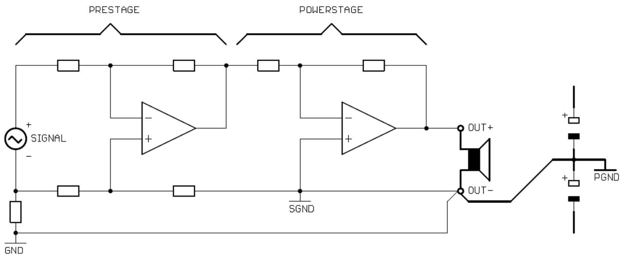
fig. 6: simplified amplifier using pseudo differential connections
