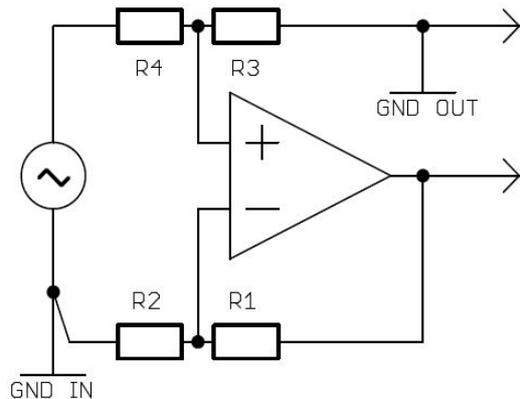
*fig.5b pseudo differential GND converter*
